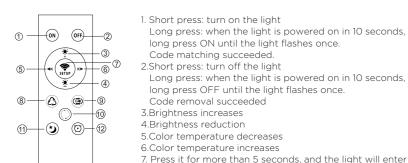
Code matching succeeded. Long press: when the light is powered on in 10 seconds, long press OFF until the light flashes once. Code removal succeeded 3.Brightness increases 4.Brightness reduction 5.Color temperature decrease
